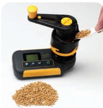
9. Hold the GrainMaster i2 against a flat and horizontal surface, and rotate the handle clockwise to grind the sample and push it through into the grain cup. If necessary, check to see the entire sample has passed through the grinder blade by turning the handle anti-clockwise a quarter turn and looking into the hopper.
